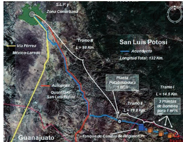
Figure 2. Sections of El Realito aqueduct
